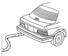
CAUTION: Be sure to use approved exhaust ventilation equipment when operating a vehicle in an enclosed area.
