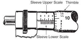
B. Reading an inside micrometer and depth micrometer is similar to reading an outside micrometer. Be sure to add the correct figure for the minimum measurement.
