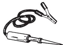
**NOTE:** The continuity light should never be used to check the power supply of electronic components.
