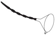
2. An oil filter removing tool is a wrench or socket adapter that fits around an oil filter to remove it.
