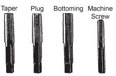
2. The sequence for cutting threads with a tap is shown below.
