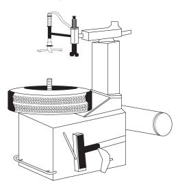
1. Its uses include removing and reinstalling the tire onto the wheel and inflating the tire to the proper pressure.
